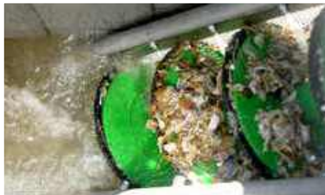
Shredded Material Moving Up the Auger Screw for Disposal
