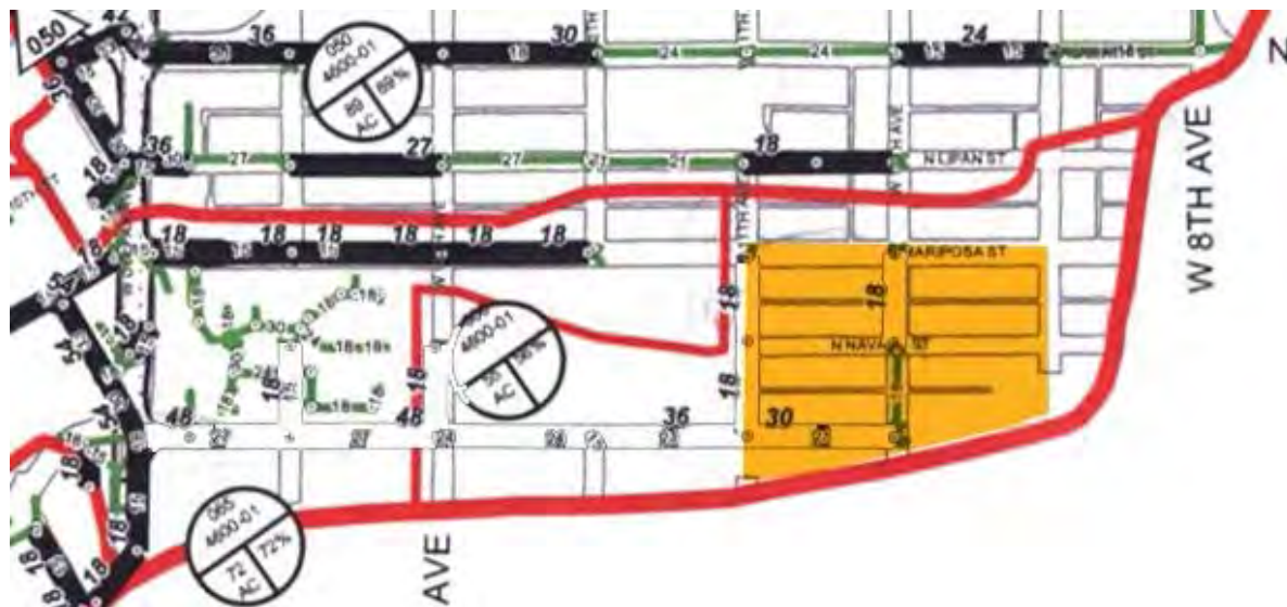
Reduced Stormwater Pipe System
