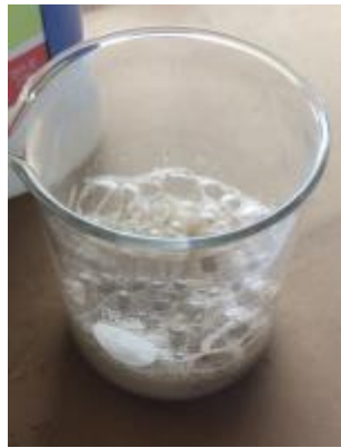
Excessive bubbling indicates a lime binder
